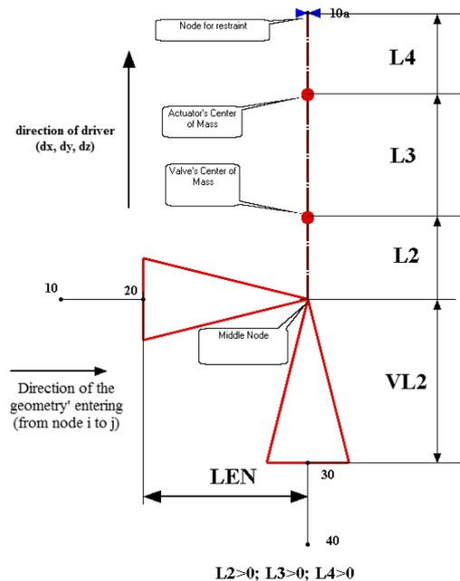
Calculation model of the angle valve
