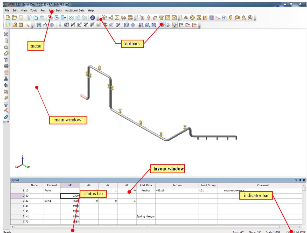
The **main window** of the program displays either the graphic model the piping system, or the model description in the form of a set of commands of the dPIPE software [input data entry language](#).
